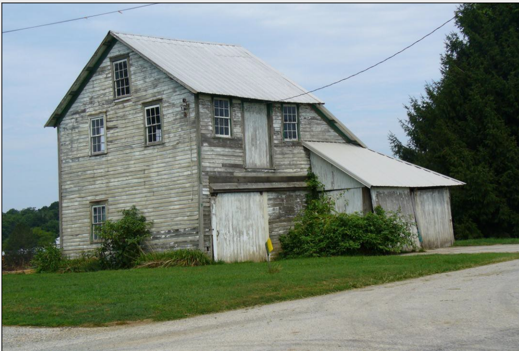
This building is located on a lane; has a well-lighted second story with loading door; has a shed roof extension which could have housed a boiler room; and is situated on a farm with a history of substantial butter production. Its identification as a creamery is not certain, but it has some important architectural characteristics associated with creamery design. Londonderry Township, Chester County, c. 1900.
