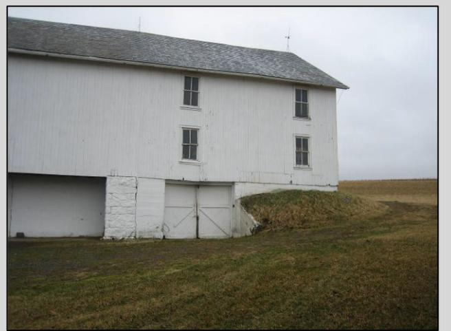
This the same barn. Its gable end was extended and a potato cellar added below; it is identifiable not only by the large doors but also by the mounded earth around the wall.
