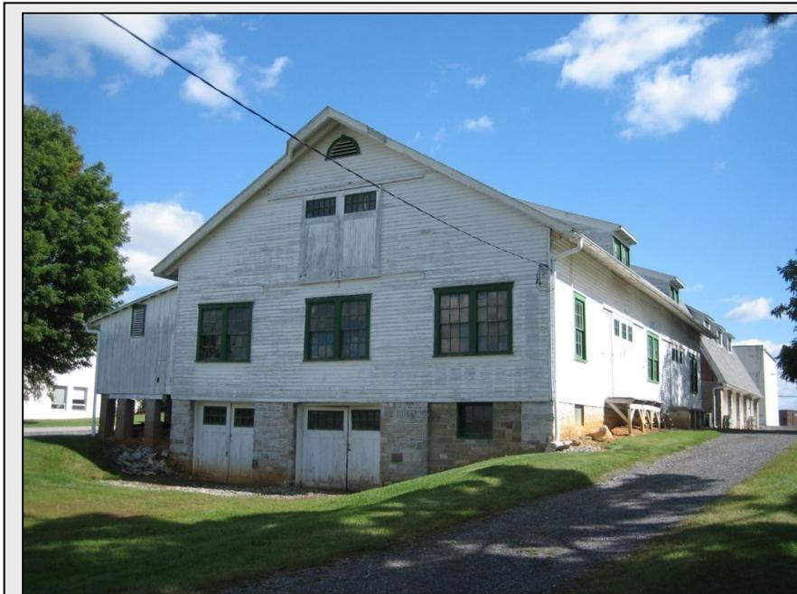
Penn State Fruit Packing House, University Park, Centre County, c 1930. Note the characteristic features: the platform with raised, sliding doors; ample interior lighting; grade-level basement entrance.
