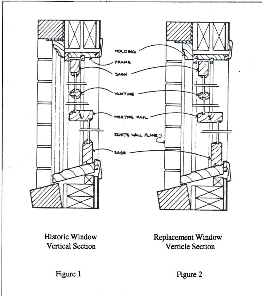
To summarize, owners are encouraged to repair the existing windows rather than replace them. If the existing condition of the window, as documented by a window survey, indicates that the window has deteriorated, then the windows may be replaced. All replacement windows will match the originals as closely as possible and must conform to the Secretary of Interior's *Standard for Rehabilitation*.
