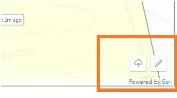
Two tools found in the lower right-hand corner of the mapping screen allow you to map the survey boundary.
