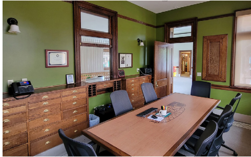
The interior of the station was both preserved and updated for modern, 21st century use. The building's important original spaces, like the stationmaster's office, lobby, and stairs, were retained, and original materials were preserved where possible. Partition walls, new doors, and new finishes were installed where needed to accommodate the building's new function.
