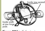
Figure MK6a. Coil-spring trap
