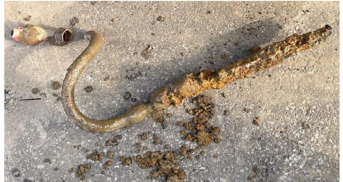
Example lead gooseneck and corroded lead service line
