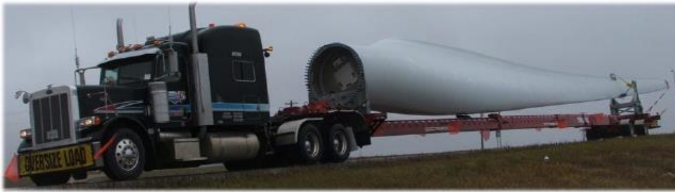
Single 45m Blade – 180 feet in Length
