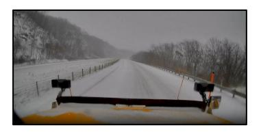
Integrating cameras, which work with the existing Geotab AVL installed in the trucks, enhances the system to provide maintenance and traffic management personnel with better situational awareness of actual road conditions during winter weather events. Video can be requested live through the system, or up to 40 hours of prior video can be requested from the digital video recorder (DVR) mounted in the truck.
