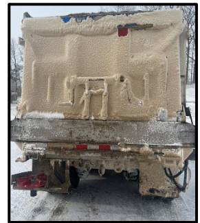
1 st Snow Event Testing Without Air Foil
