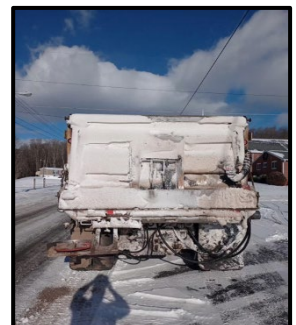
2 nd Snow Event Testing Without Air Foil
