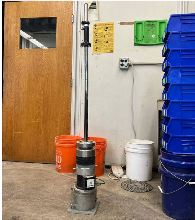
Figure 35. LWD in the compacted soil in the Proctor mold.
