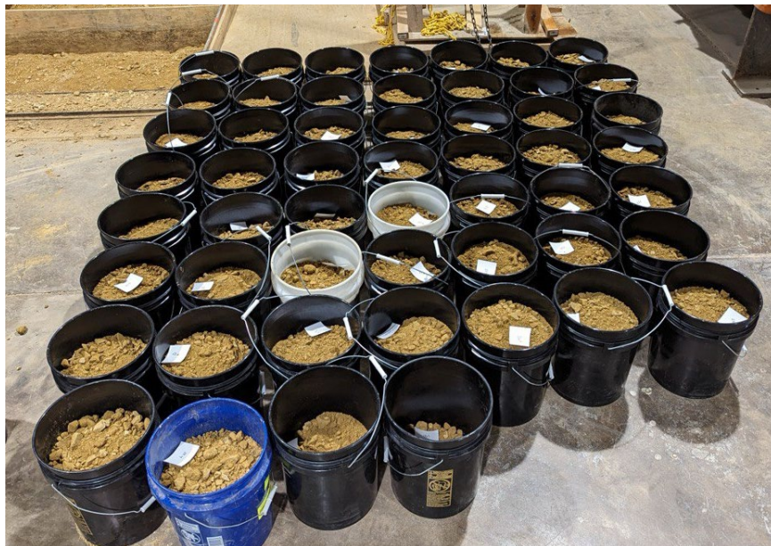
Figure 40. Soil prepared for placement in the test pit before testing.
