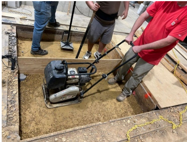
Figure 30: The vibratory plate compactor used in this study.
