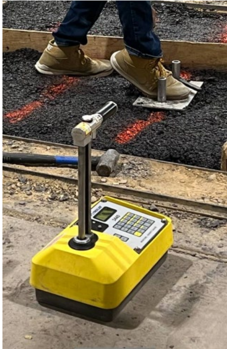
Figure 31 Nuclear Moisture-Density Gauge used in this study.
