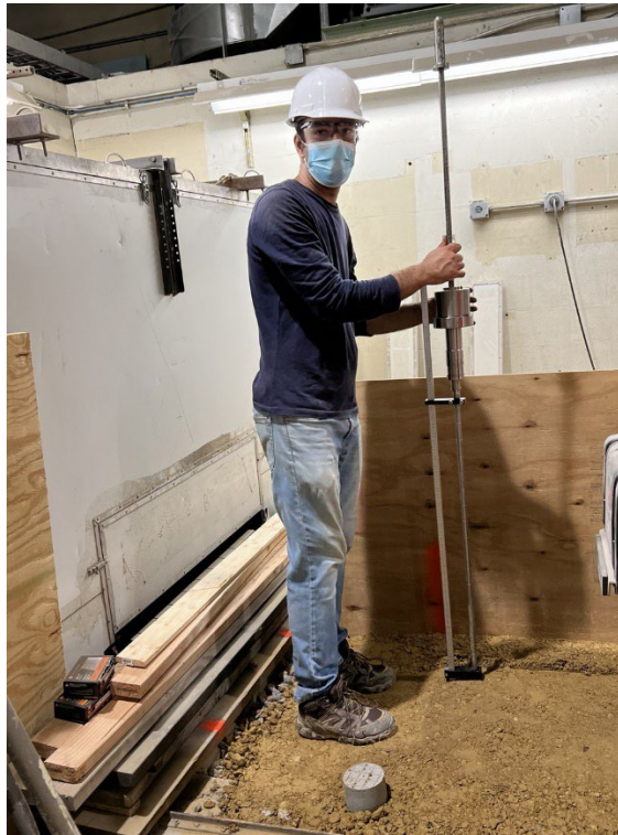
Figure 33. The DCP used in this study.
