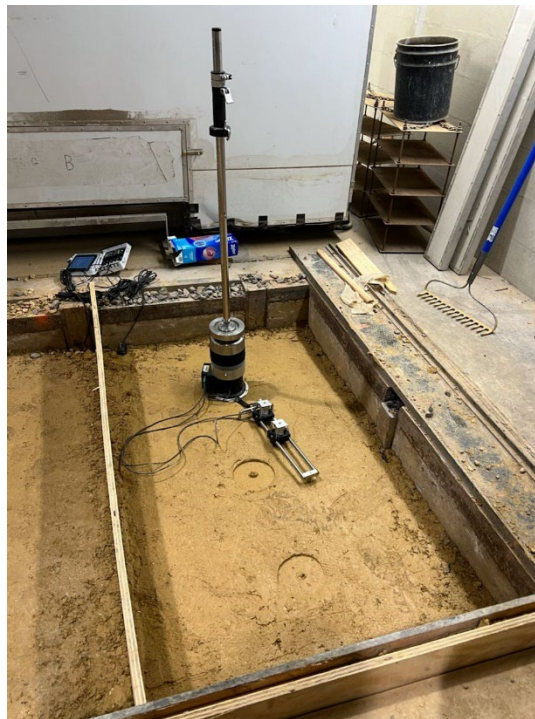
Figure 32: The LWD used in this study.
