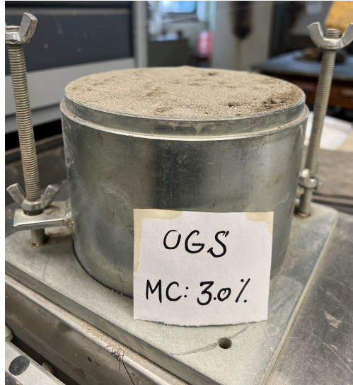
Figure 34. A Compacted Soil Specimen with fine sand applied to the surface.
