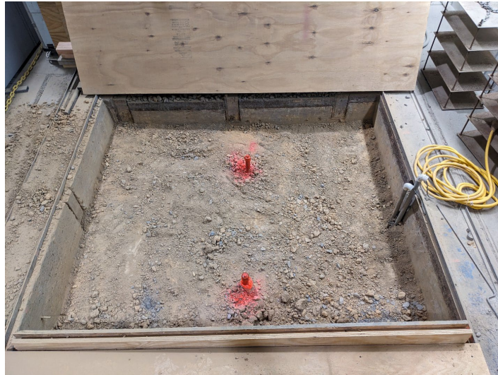
Figure 39. The existing soil after removal of the topsoil and before placement of the soil to be tested (anchors were also removed).
