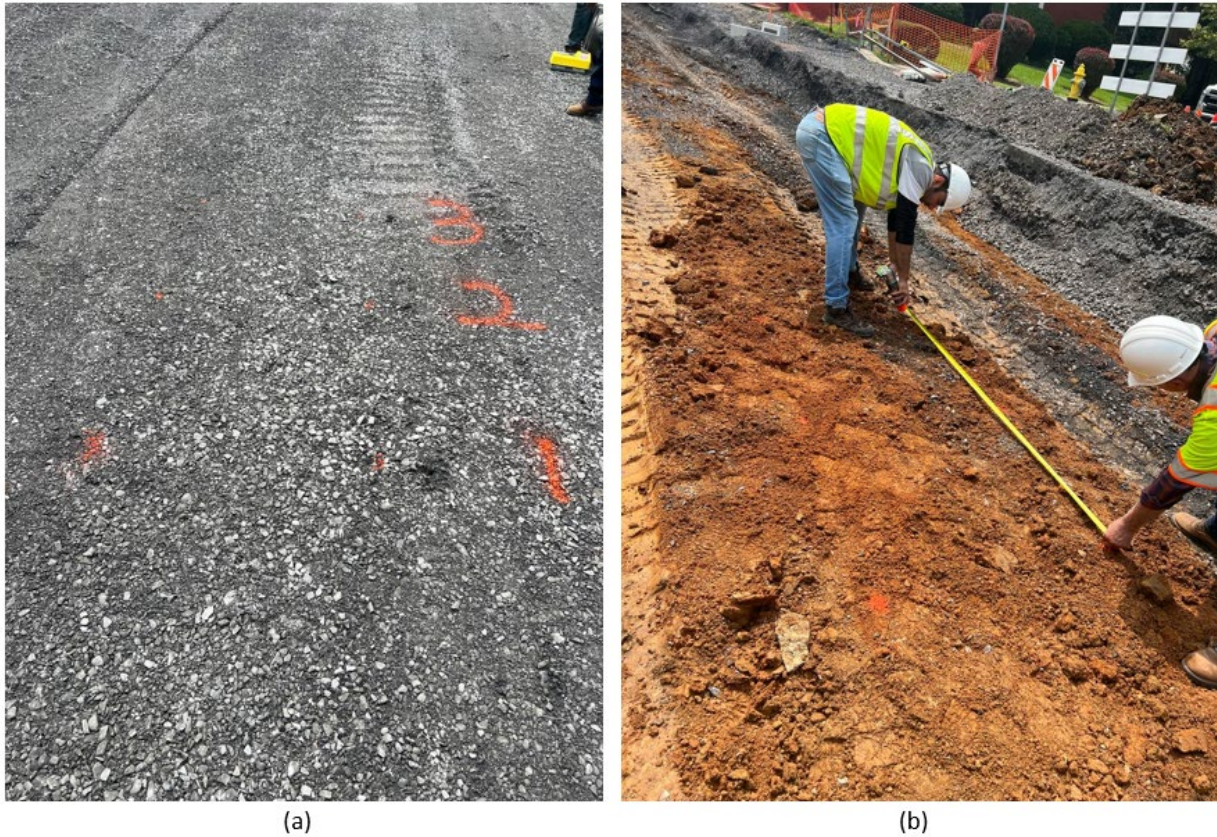
Figure 45. Determination of three spots 3 ft apart longitudinally at: (a) 2A and (b) A6 materials.
