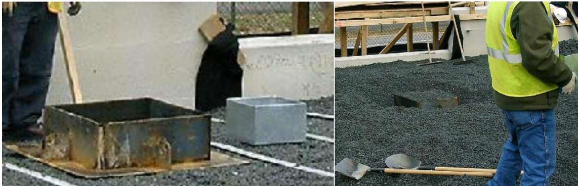
Figure 4.38. Quality control of compaction efforts for ESCS based on steel boxes (Left) removed after compaction (Right).
