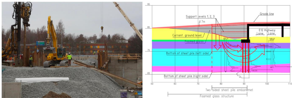
Figure 1.38. Auvinen et al. (2013) FWG case history: (left) longitudinal section of the foamed glass ramp onto concrete shell of tunnel; (Right) foamed glass embankment during construction.
