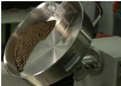
a) Paste into pelletizer's pan
