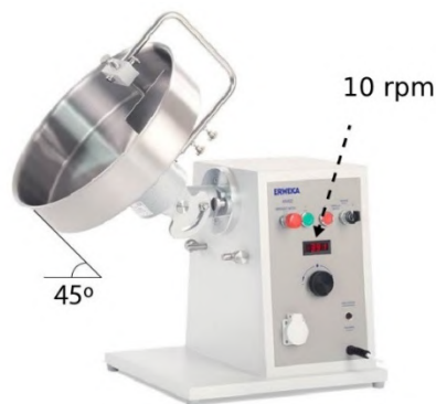
Figure 15. Pelletizer with adjusted angle 45° and set speed 10 rpm.
