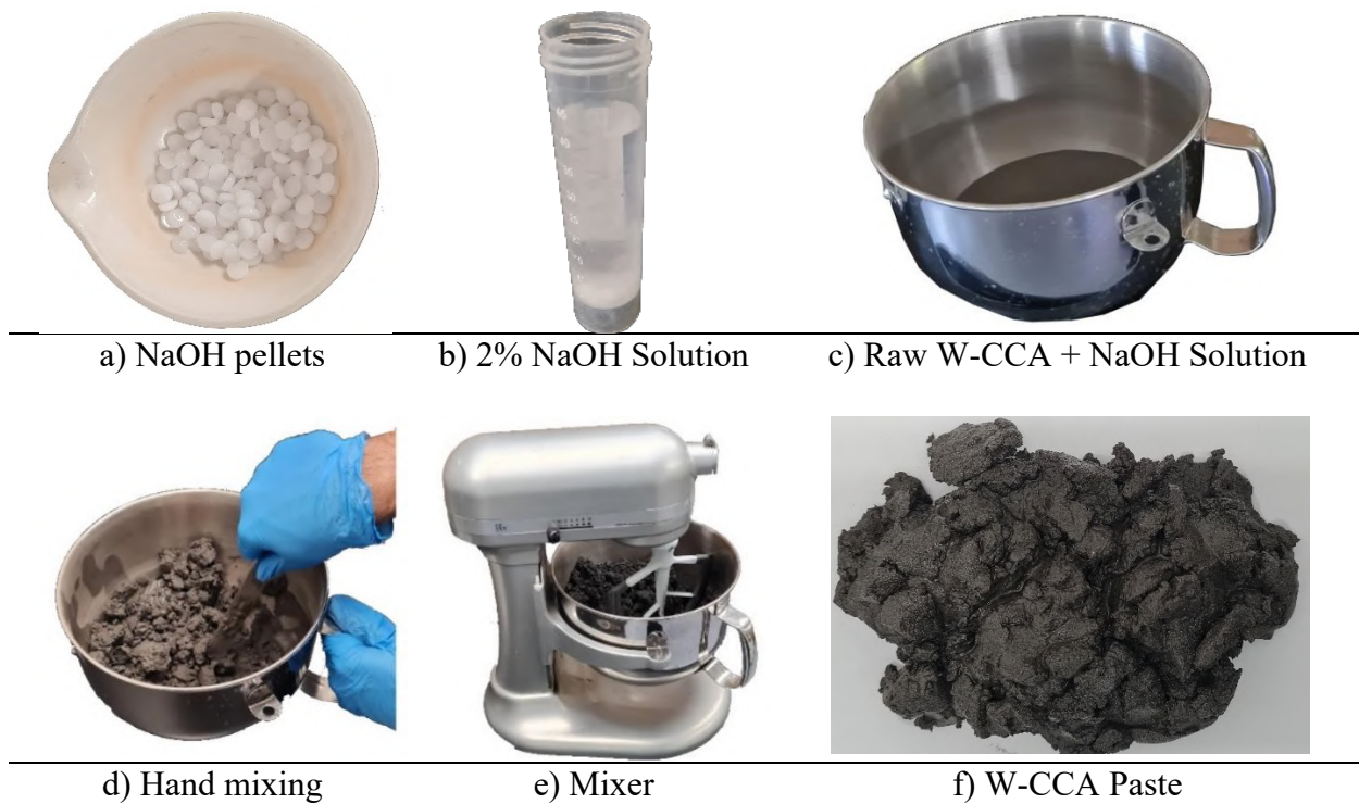
Figure 14. Phase 1: W-CCA paste preparation.
