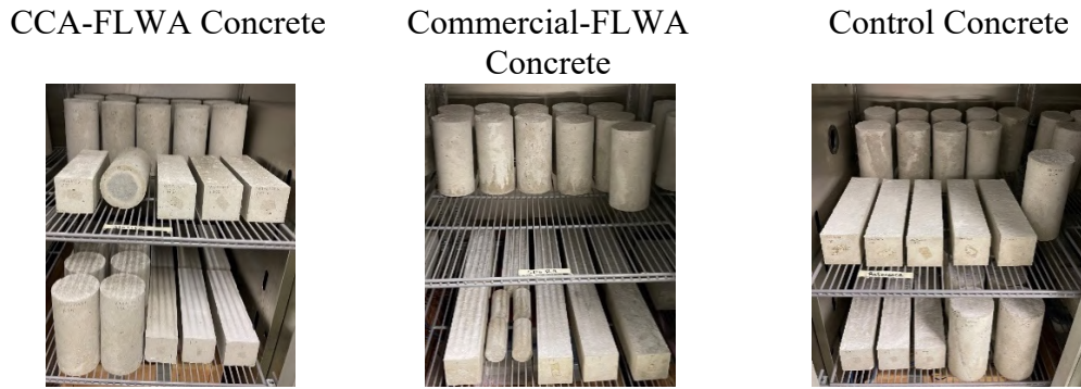
Figure 39. Concrete cast specimens for CCA-FLWA, Commercial-FLWA, and control concrete.
