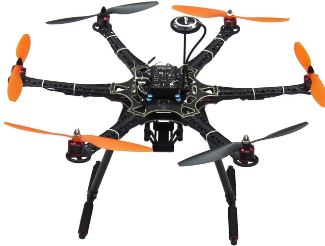
Figure 2.4. DIY Drone based on the Generic S550 Frame
