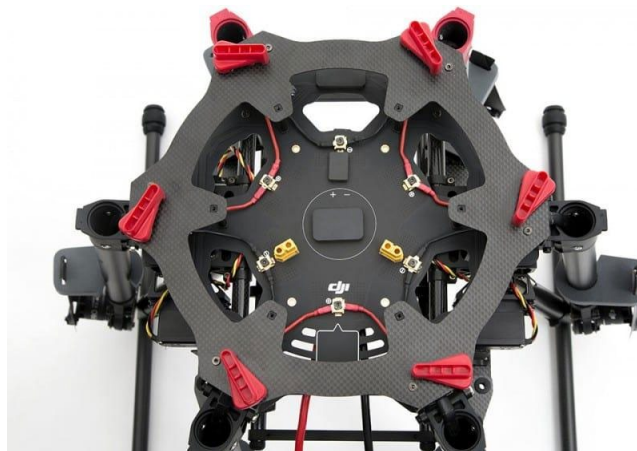
Figure 6. Frame Integrated Power Distribution Board from a DJI S900
