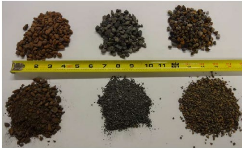
Figure 2-5 From left to right: Expanded shale, expanded slate, expanded clay; from top to bottom: coarse aggregates and fine aggregates (from Krc 2015).
