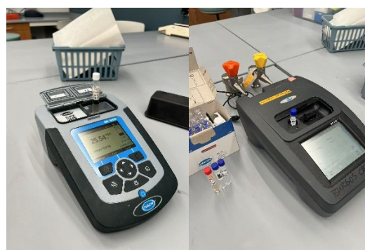
(b) Hach DR 1900 and 2800 spectrophotometers
