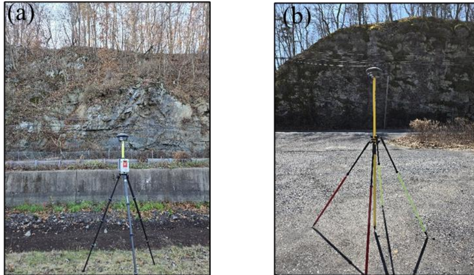
Figure 113. Scan equipment (a) RTC 360 scanner with rover mounted on top (b) GS18 set up as a base station.
