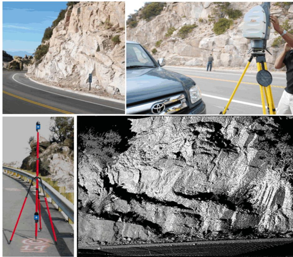
Figure 6. Scanning rock slopes adjacent to highways with the Leica ScanStation; Point cloud is shown in the bottom right (Kenemy and Turner 2008).
