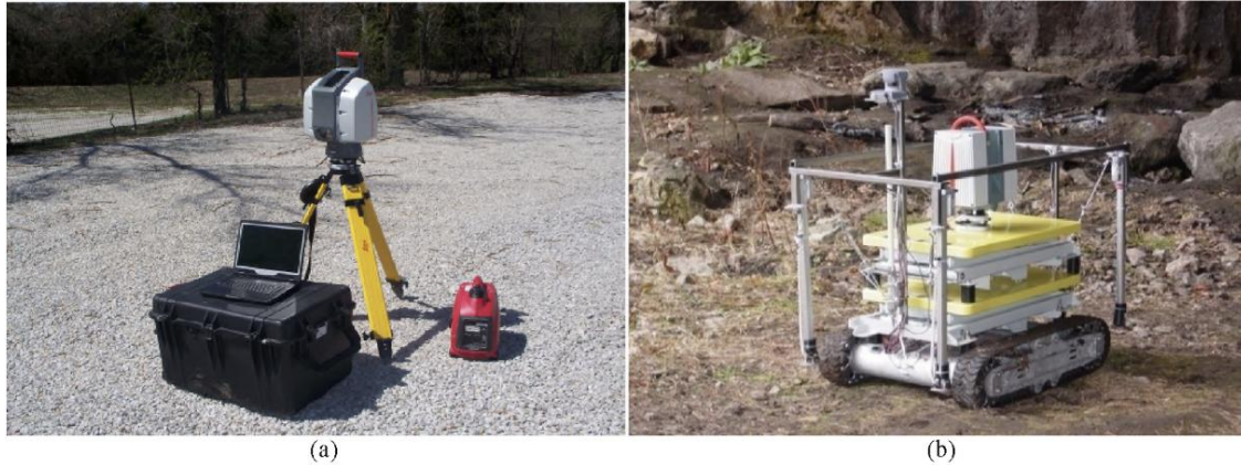
Figure 4. (a) Leica ScanStation II time of flight scanner with integrated optical camera; (b) Leica HDS 6000 phase shift scanner (adopted from Maerz et al., 2015).
