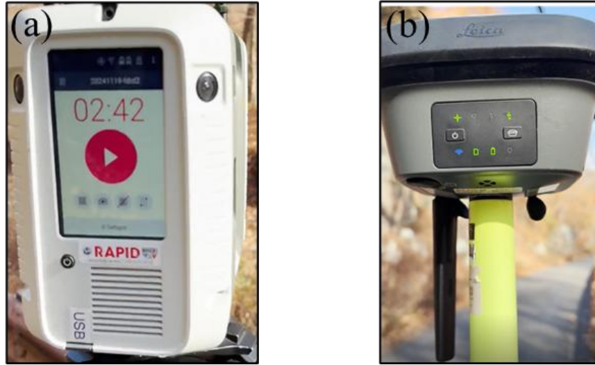
Figure 115. (a) RTC360 scanner screen display showing scan settings (b) GS18 controller status.
