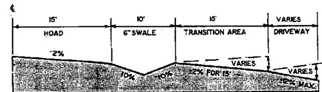
NOTE DRIVEWAYS FOR INDIVIDUAL LOTS SHALL CONFORM TO THE SPECIFICATIONS OF THIS TYPICAL DRIVEWAY SECTION & OF DRIVEWAYS SHALL BE LOCATED AT LEAST 75' FROM & OF ROAD INTERSECTION.
