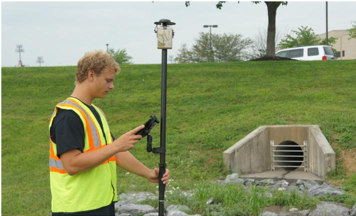
Jake Holbert of Land Logics Group uses Collector for ArcGIS and the Arrow 100 for collecting stormwater asset data in the field.
