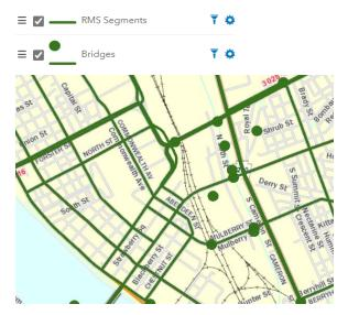
State roads and bridges can be added to your project area through the **Layer Information** box or the **Lasso Tool**. To add a road or bridge using the **Layer Information** box, first close the Redline Tool box, then click on a route segment or bridge on the map.
