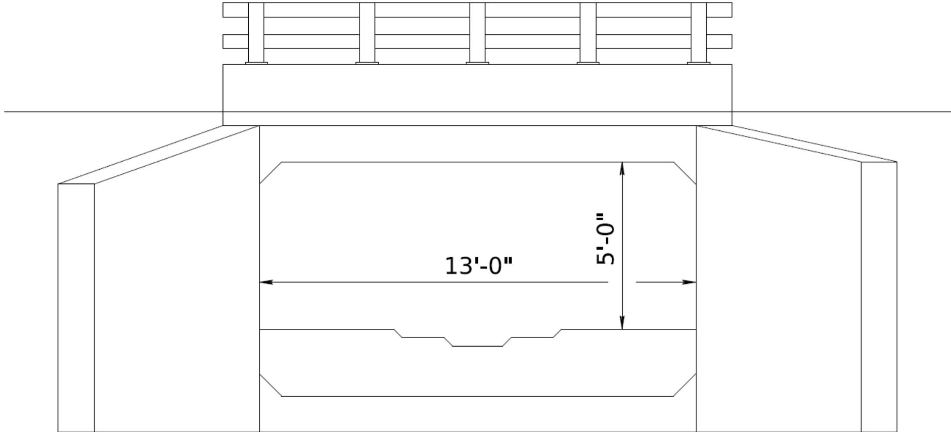
**PRECAST CONCRETE BOX CULVERT**
