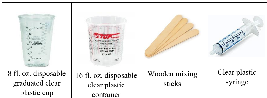
Figure 2: Typical Lab Supplies for Preparing Tensile Test Specimens from Binder Resin.
