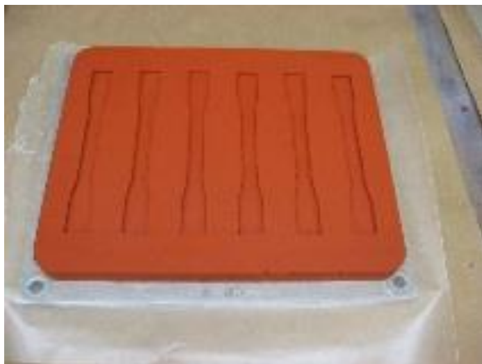
Figure 1: Typical silicone mold for forming Type I Dumbbell-Shaped Tensile Test Specimens.
