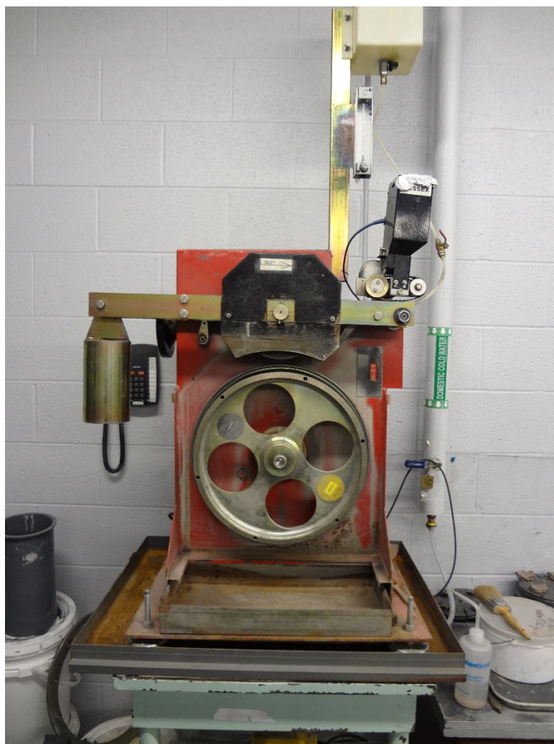
Figure 1- Accelerated Polishing Machine with a Specimen Wheel Cover Removed
