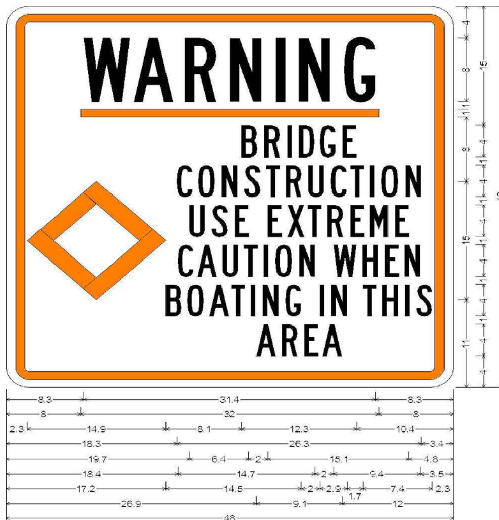
FIGURE 10.5.1 EXAMPLE OF ATON SIGN SPECIFICATION FOR PLACEMENT UPSTREAM AND DOWNSTREAM OF PROJECT AREA
