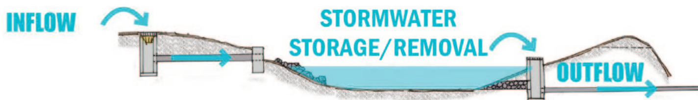
Figure 1.4.1: Stormwater Runoff- SCM Process
