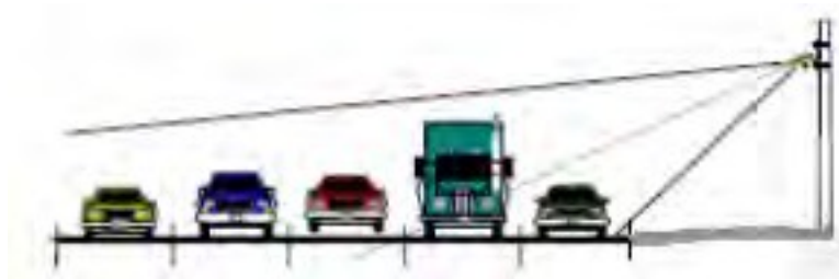
FIGURE 16: MICROWAVE/RADAR DETECTOR ORIENTATION
