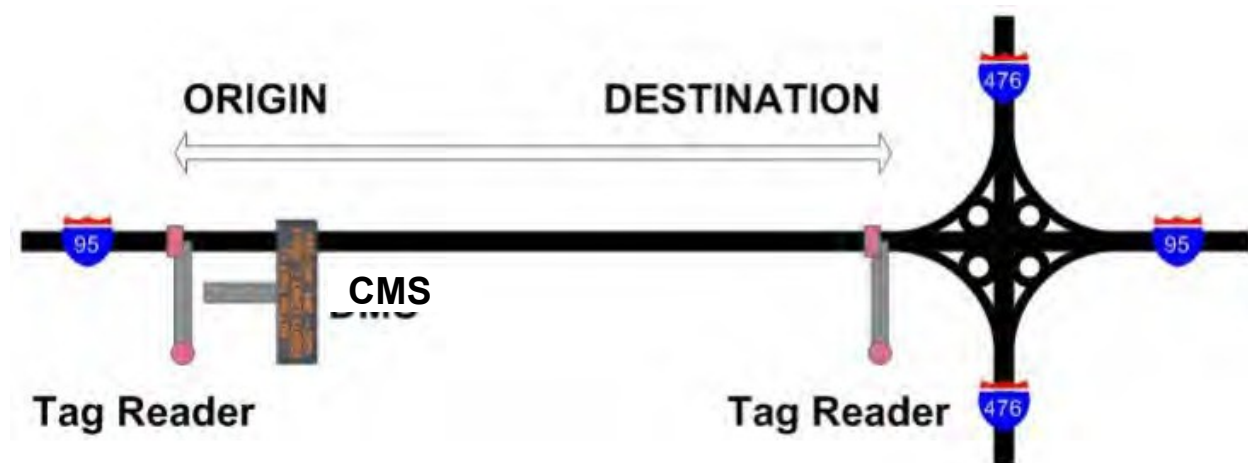
FIGURE 25: ORIGIN-DESTINATION TRAVEL TIME SYSTEM LAYOUT
