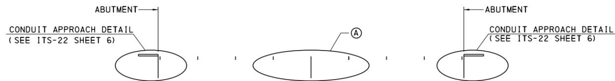
**CONDUIT SUPPORT CONFIGURATION: SINGLE SPAN BRIDGE**
