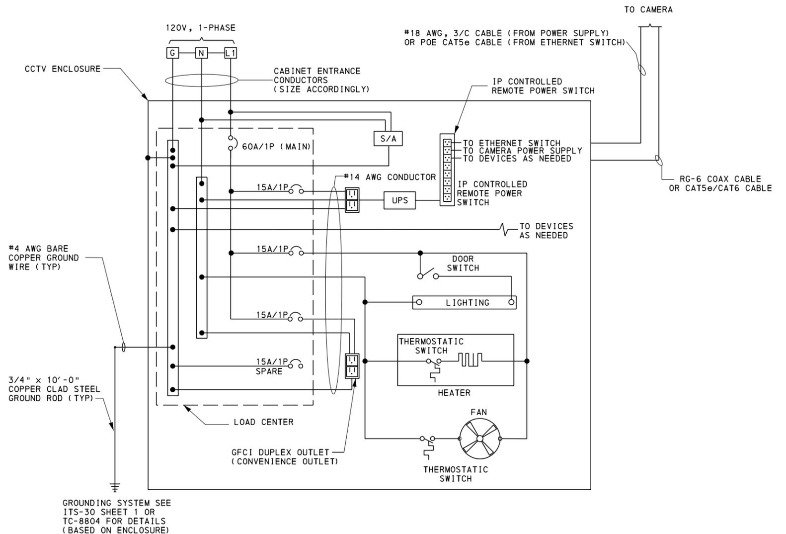
**TYPICAL CCTV WIRING DIAGRAM**
