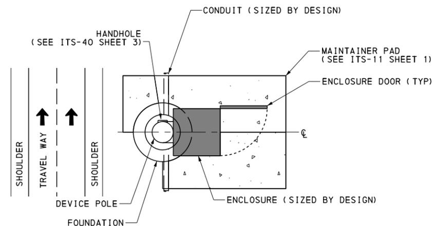
**POLE MOUNTED ITS ENCLOSURE ORIENTATION
