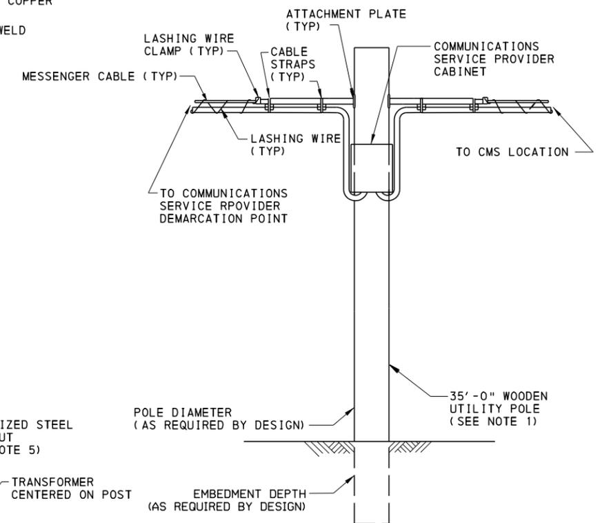
**WOODEN UTILITY POLE ELEVATION FOR CMS LOCATIONS (BACK VIEW)**
