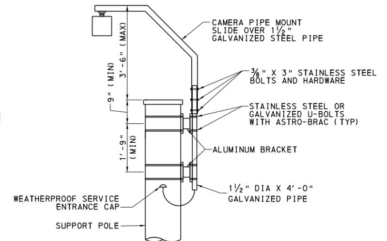
CCTV CAMERA ATTACHMENT TO EXISTING TRAFFIC SIGNAL STRUCTURE
