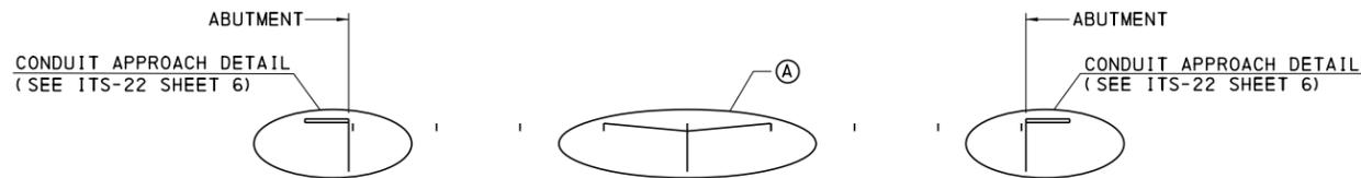
**CONDUIT SUPPORT CONFIGURATION: SINGLE SPAN BRIDGE**
