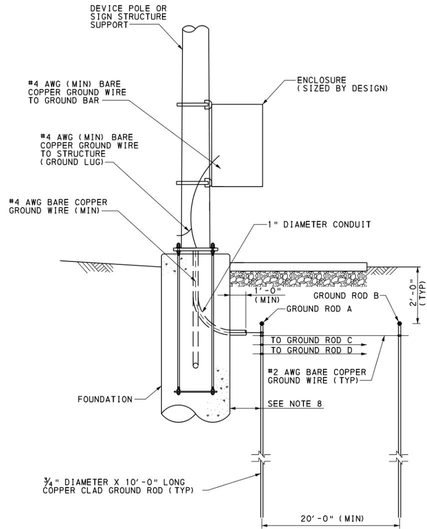
**GROUNDING DETAIL FOR POLE AND STRUCTURE MOUNTED ITS ENCLOSURE**
