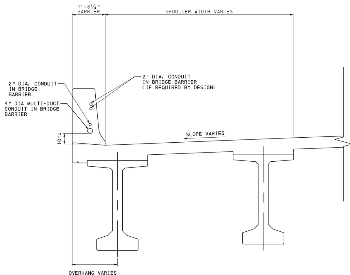
CONDUIT IN BRIDGE BARRIER DETAIL
