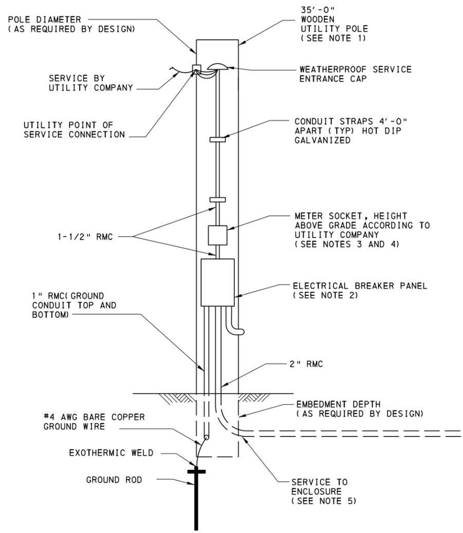
**WOODEN UTILITY POLE ELEVATION (FRONT VIEW)**
