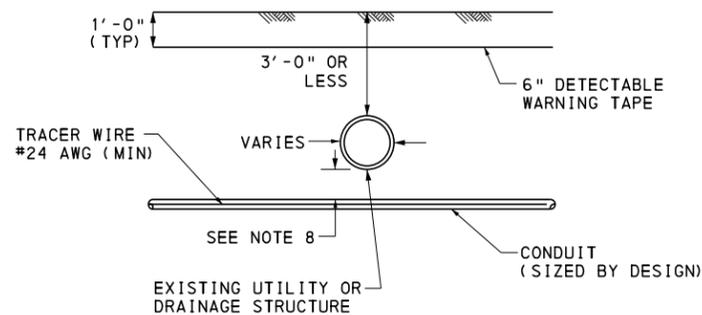
**CONDUIT INSTALLATION DETAIL BELOW
