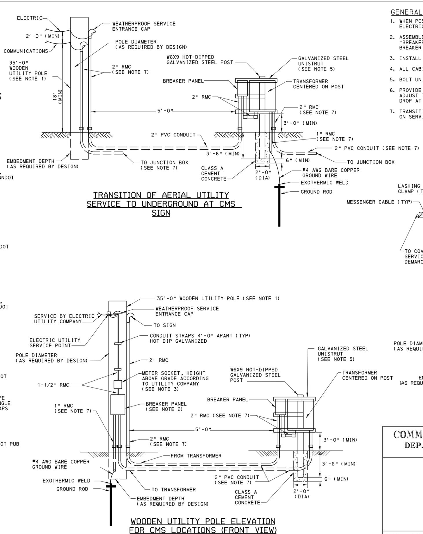
**WOODEN UTILITY POLE ELEVATION FOR CMS LOCATIONS (FRONT VIEW)**
