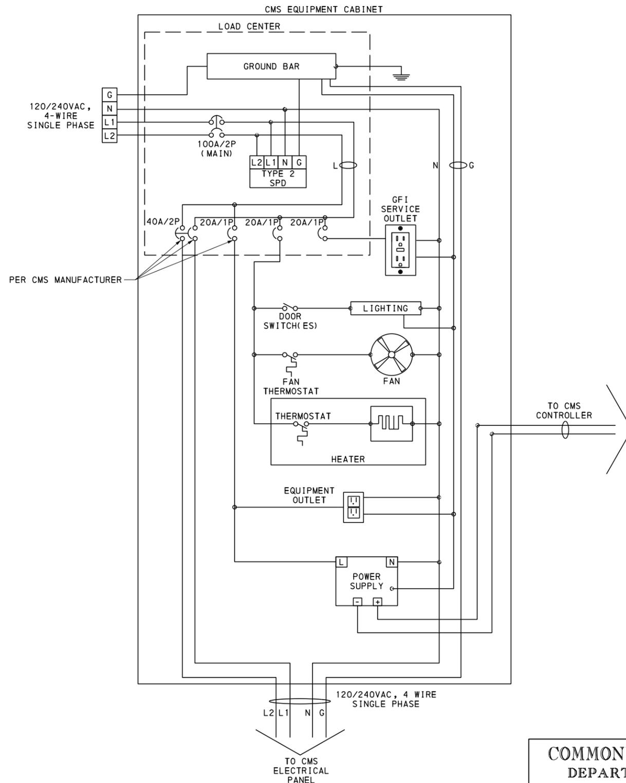
**TYPICAL CMS WIRING DIAGRAM**
