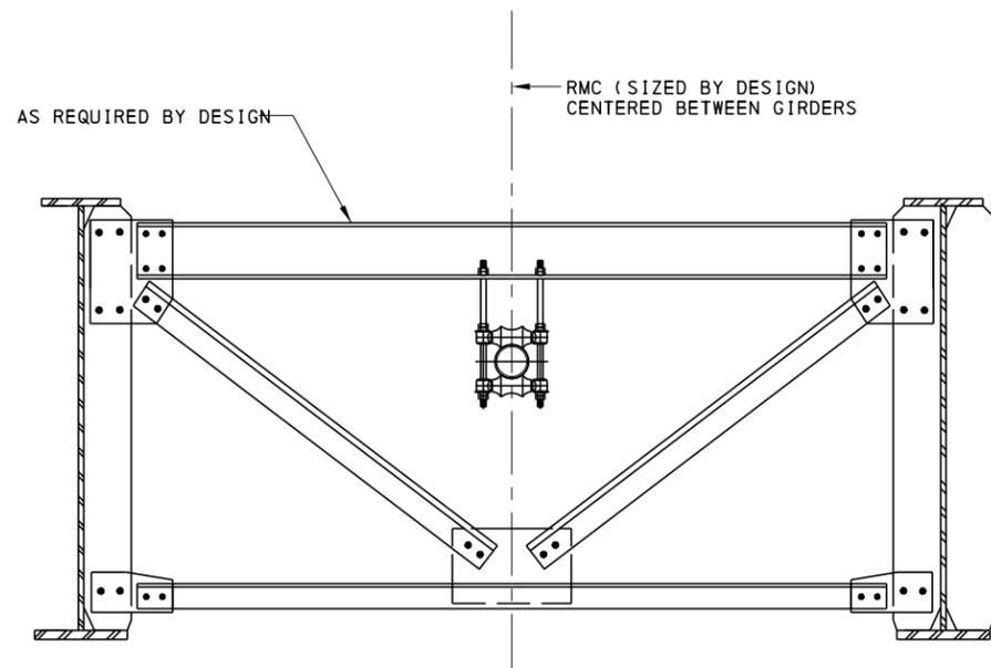
**TYPICAL INTERMEDIATE DIAPHRAGM CONDUIT SUPPORT DETAIL**
