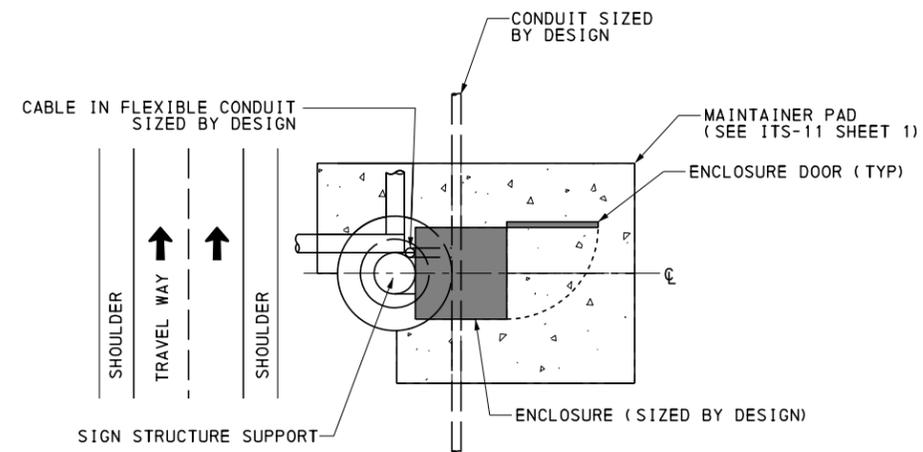
**STRUCTURE MOUNTED ITS ENCLOSURE ORIENTATION
