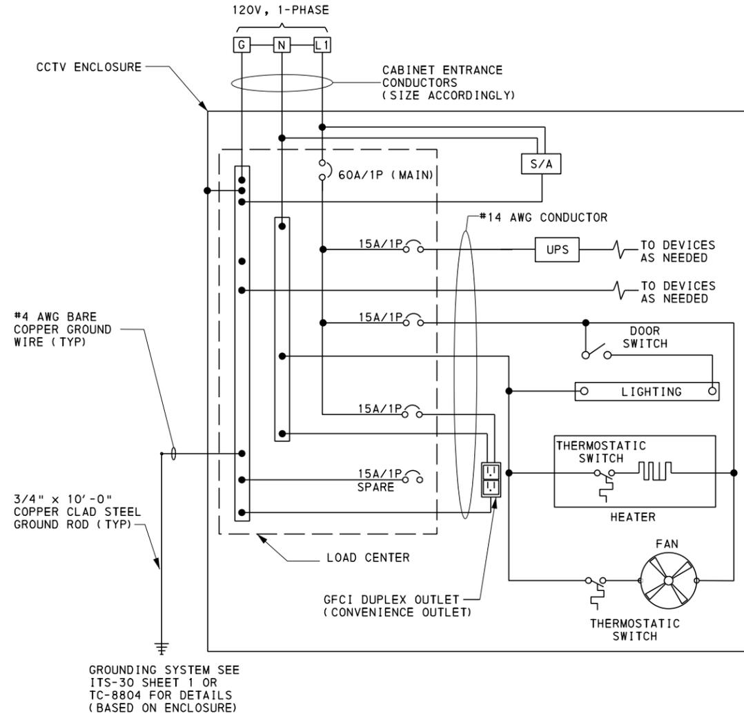
**TYPICAL HUB WIRING DIAGRAM**
