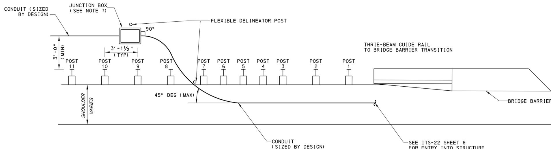
**BRIDGE APPROACH END CONDUIT DETAIL (PLAN VIEW)**
