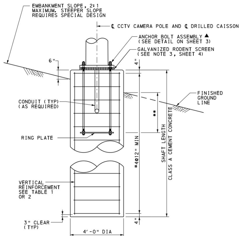
**DRILLED CAISSON ELEVATION**
