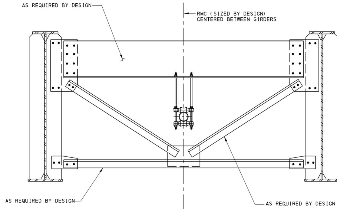
**TYPICAL END DIAPHRAGM CONDUIT SUPPORT DETAIL**
