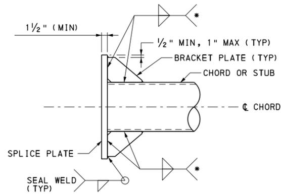
**CHORD SPLICE ASSEMBLY WELD DETAIL**
