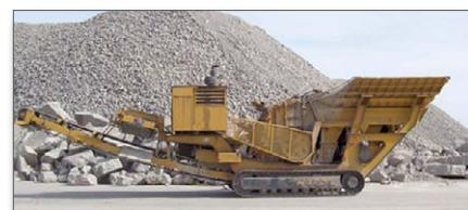
**Figure 6. Crushed concrete stockpile and crusher**
