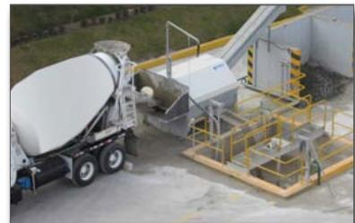
**Figure 5. Ready mixed truck washing out into a reclaimer**
