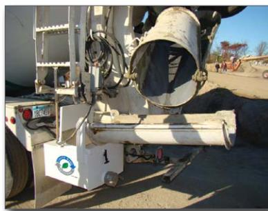
Figure 7. Chute washout box
