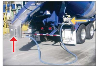
Figure 8. Chute washout bucket and pump
