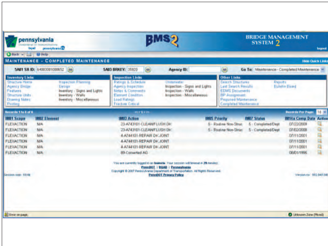
Figure 6-9 – Closing a Work Order in BMS Web Completed Maintenance Screen
