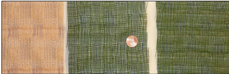
Figure 14.3.7.1-3 – Deformed Synthetic Three-dimensional Turf Reinforcement Mats
