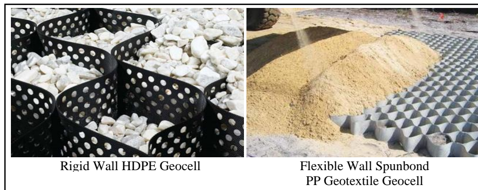
Figure 14.3.4-1 – Typical Geocell (Typical Application – Load Distribution)
