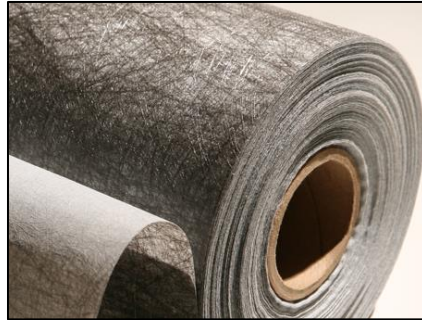
Figure 14.3.1.5-1 – Typical NW-SB Geotextile PP (Typical Application – Separation)
