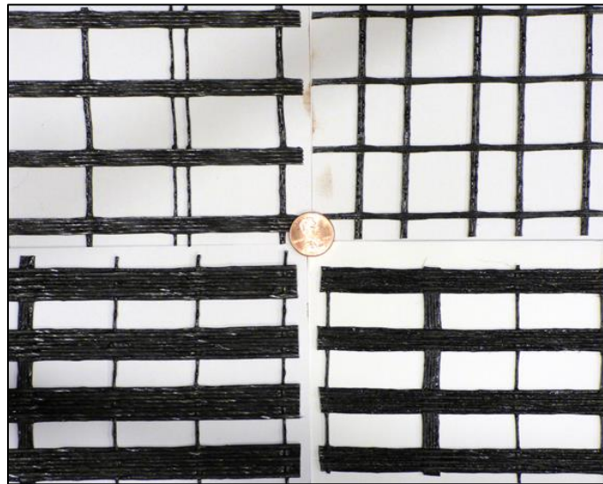
Figure 14.3.2.1-1 – Woven/Knitted Uniaxial Geogrid (Typical Application – Reinforcement)
