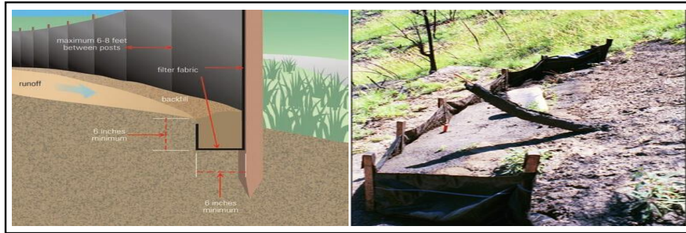
Figure 14.3.1.2-2 – Typical Silt Fence Installation
