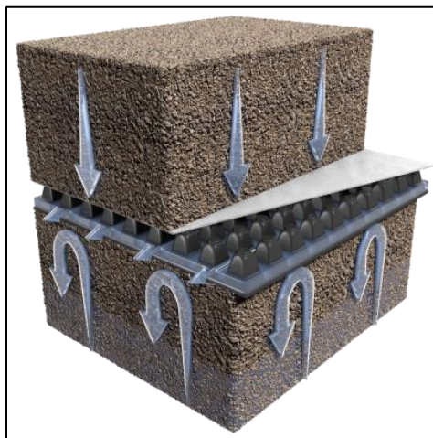
Figure 14.7.2-1 – Schematic of Geosynthetic Drainage Composite as a Capillary Break
