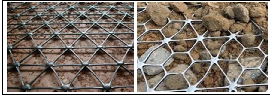
Figure 14.3.2.3-1 – Integrally Formed Punched Drawn Multi-Axial Geogrids (Typical Application – Stabilization)
