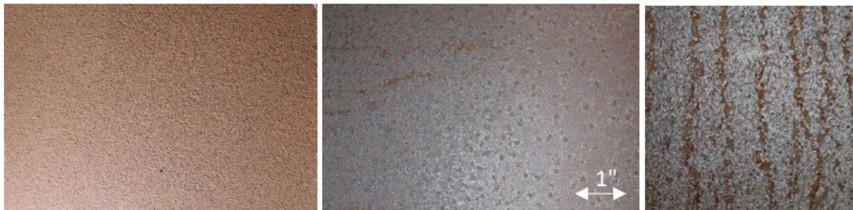
Figure 10 – Views of good-performing UWS showing a smooth surface of varying colors (Source: NSBA/AISC 2022)
