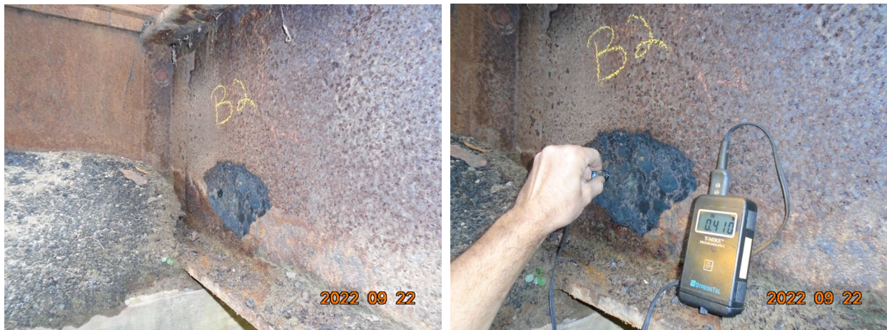
Figure 17 – Views of Cleaned Surface and Ultrasonic Testing Gauge Measurement
