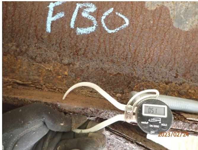
Figure 16 – View of Thickness Measurement with a Digital Caliper
