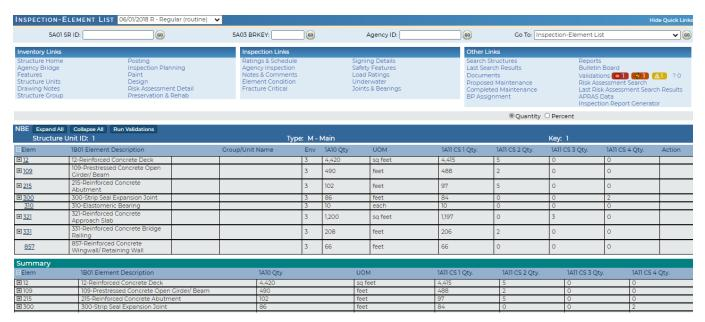
Figure 2.5.5.1-1 Element Condition Screen
