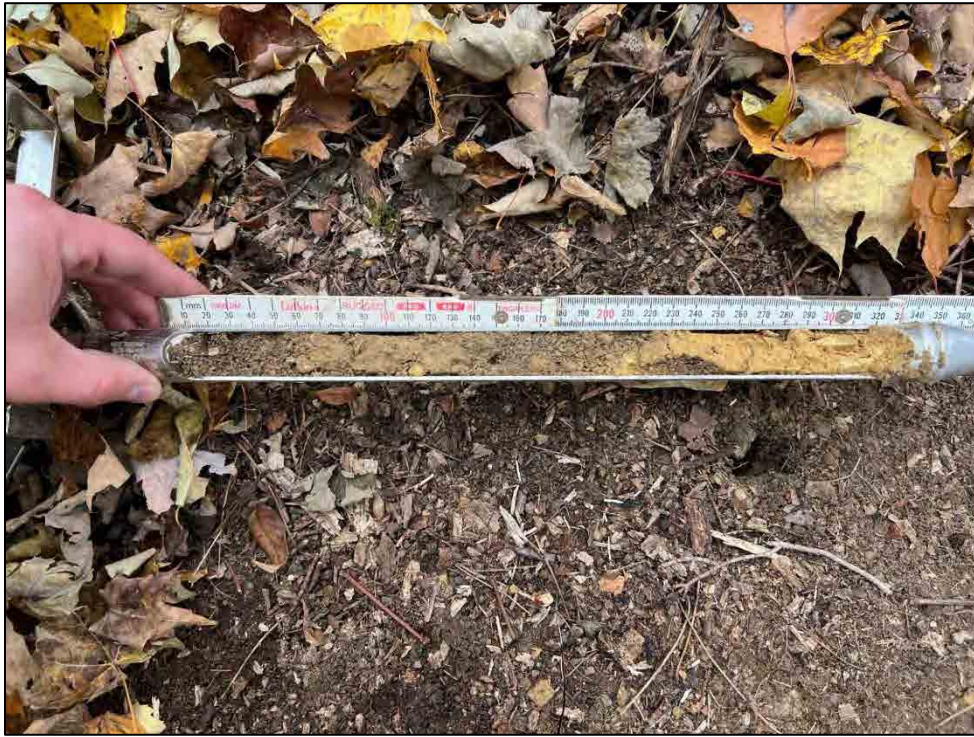
Photograph 19: Upland soil profile in Boring 4, retrieved from eastern terrace along WL014 near its source. Photograph taken October 18, 2022.
