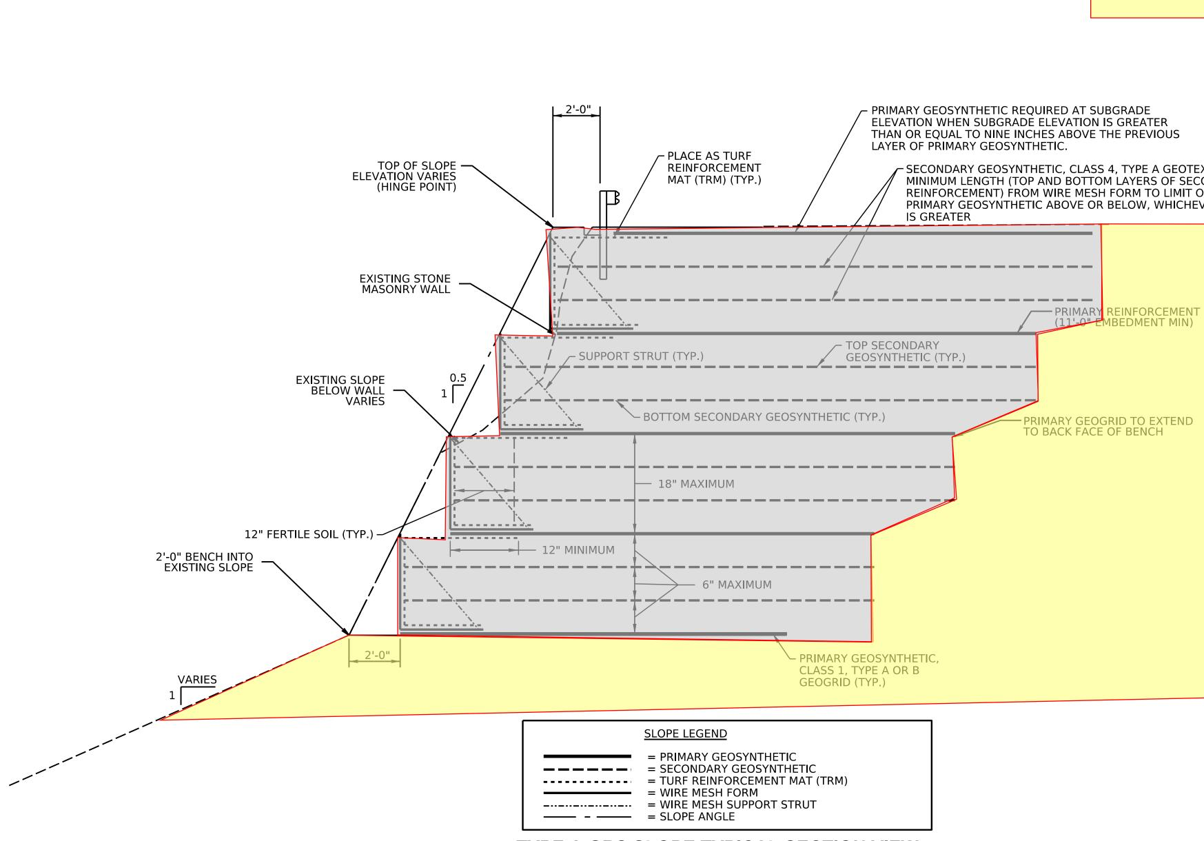
**TYPE A GRS SLOPE TYPICAL SECTION VIEW**
