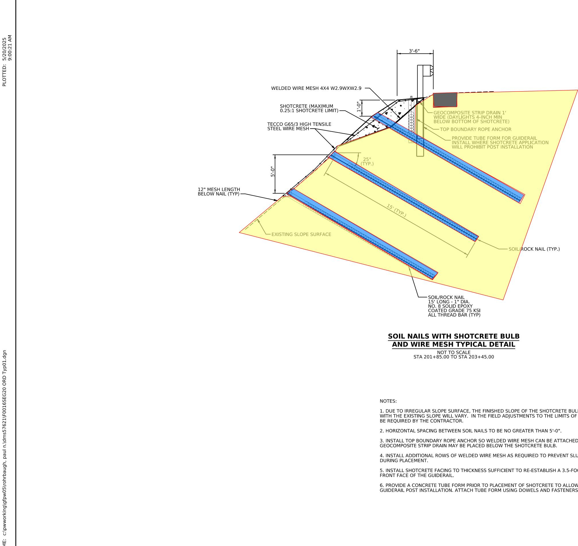
1. DUE TO IRREGULAR SLOPE SURFACE, THE FINISHED SLOPE OF THE SHOTCRETE BULB AND LOCATION IT MEETS WITH THE EXISTING SLOPE WILL VARY. IN THE FIELD ADJUSTMENTS TO THE LIMITS OF THE SHOTCRETE BULB WILL
