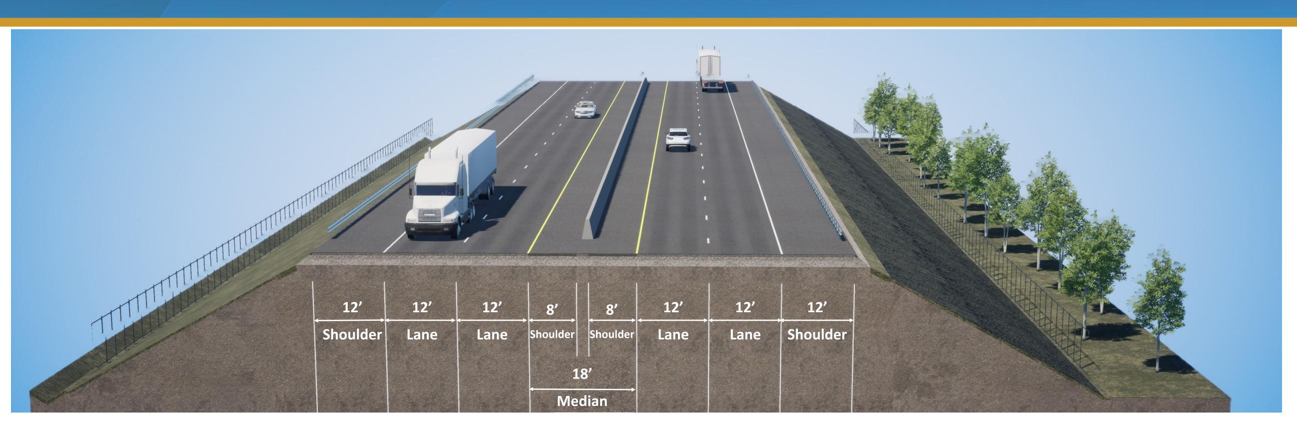
Section used at western and eastern ends of the Build Alternative
