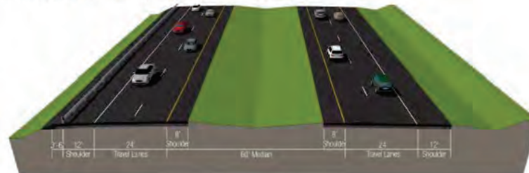
60-Foot Median Typical Section – Original
