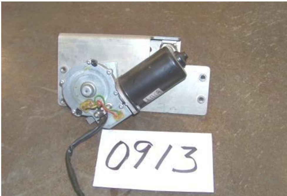
WIPER MOTOR REMOVAL AND REPLACEMENT (0.5 MAN HOURS)
