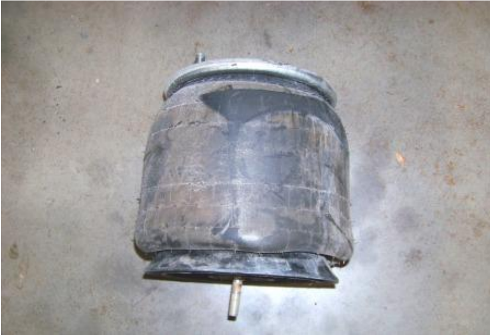
LEAKING LEFT FRONT AIR BAG (1,591 TEST MILES)
