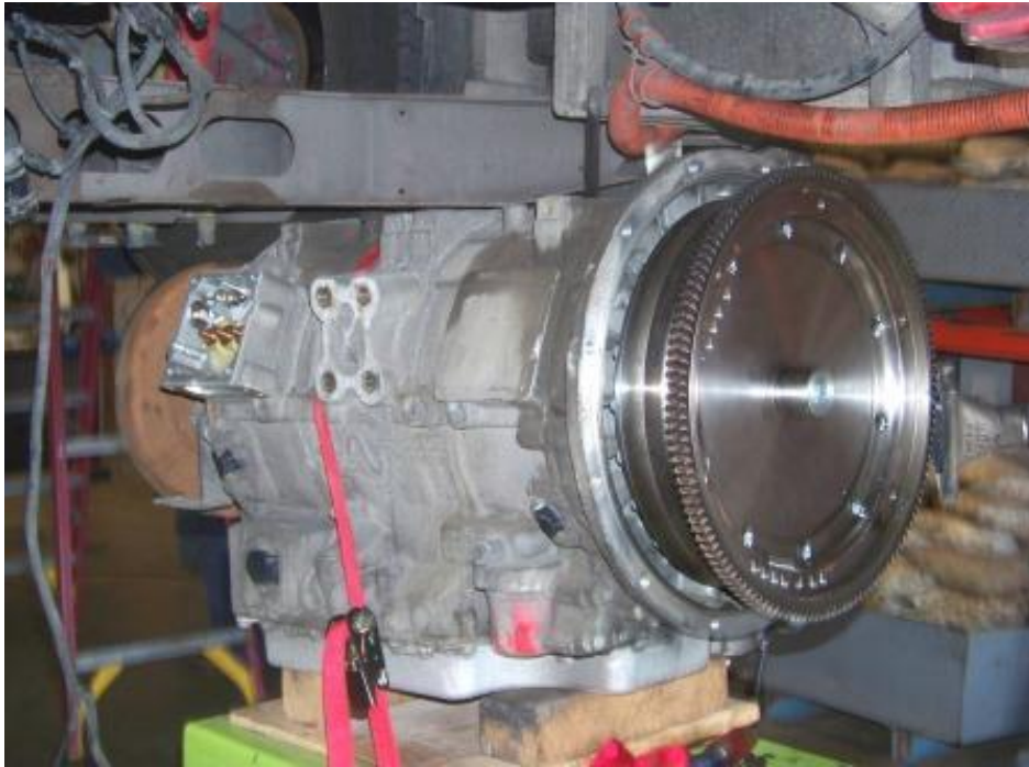
TRANSMISSION REMOVAL AND REPLACEMENT (18.0 MAN HOURS)
