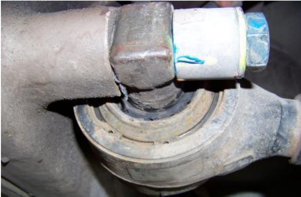
WORN BUSHING; RIGHT FRONT LOWER RADIUS ROD (4,273 TEST MILES)
