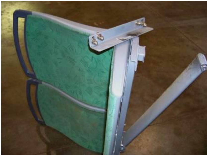
FAILED SEAT BRACKET (7,751 TEST MILES)
