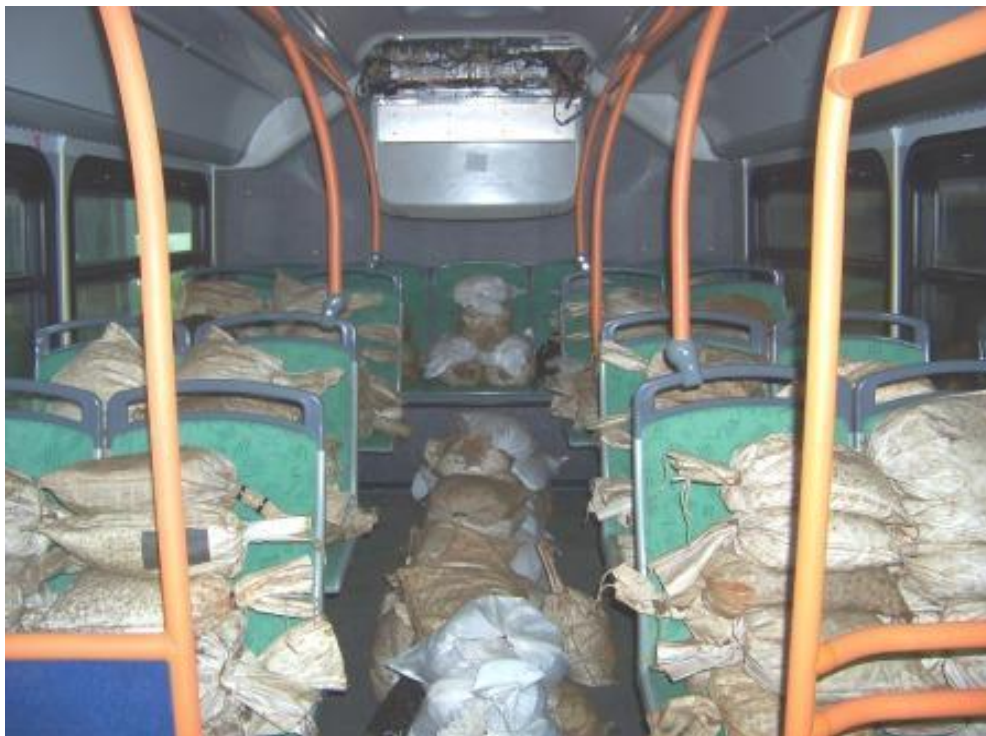
BUS LOADED TO 2.5 TIMES GVW (31,125 LBS)
