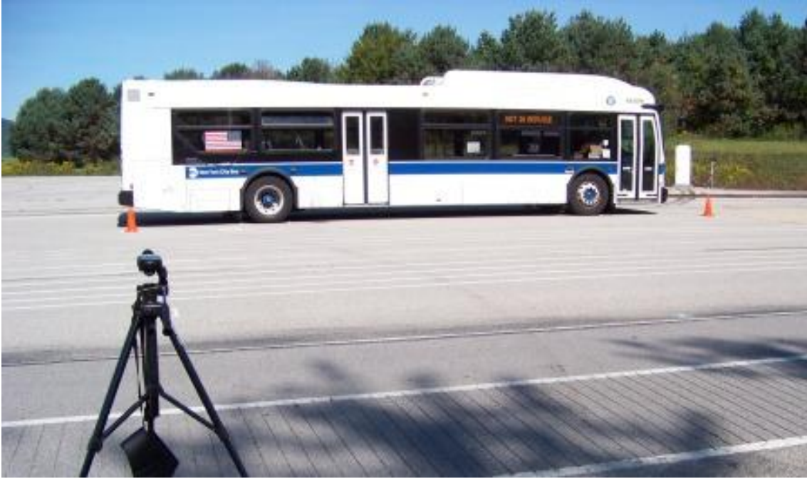
TEST BUS UNDERGOING EXTERIOR NOISE TESTING
