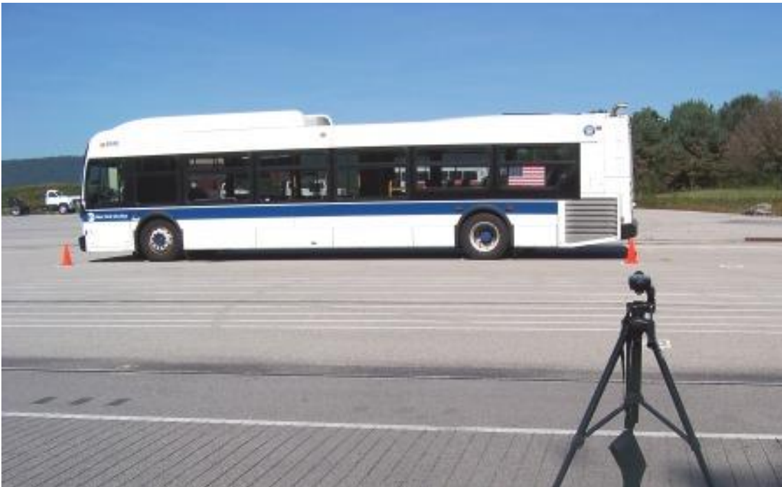
TEST BUS UNDERGOING EXTERIOR NOISE TESTING
