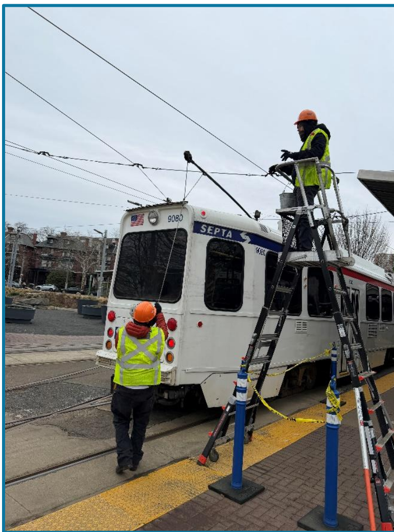
Image 8. SEPTA Trolley Slider Inspection. March 18, 2026.
