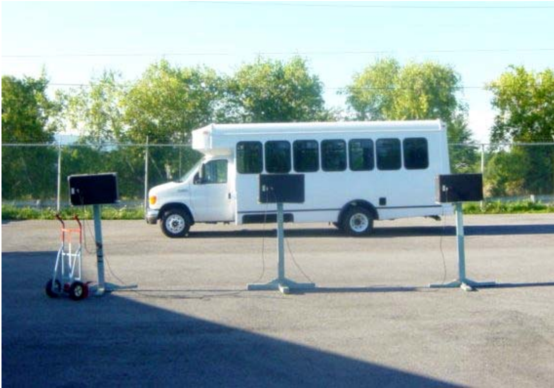
TEST BUS SET-UP FOR 80 dB(A) INTERIOR NOISE TEST
