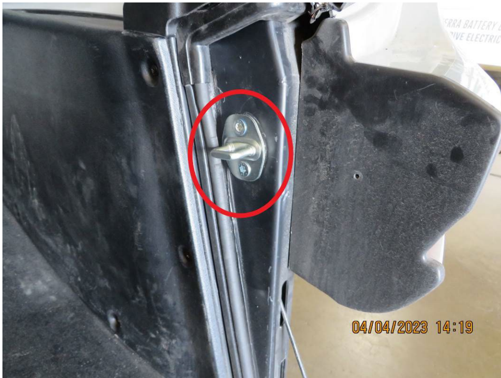
REPLACED REAR DOOR LATCH (3,701 TEST MILES)
