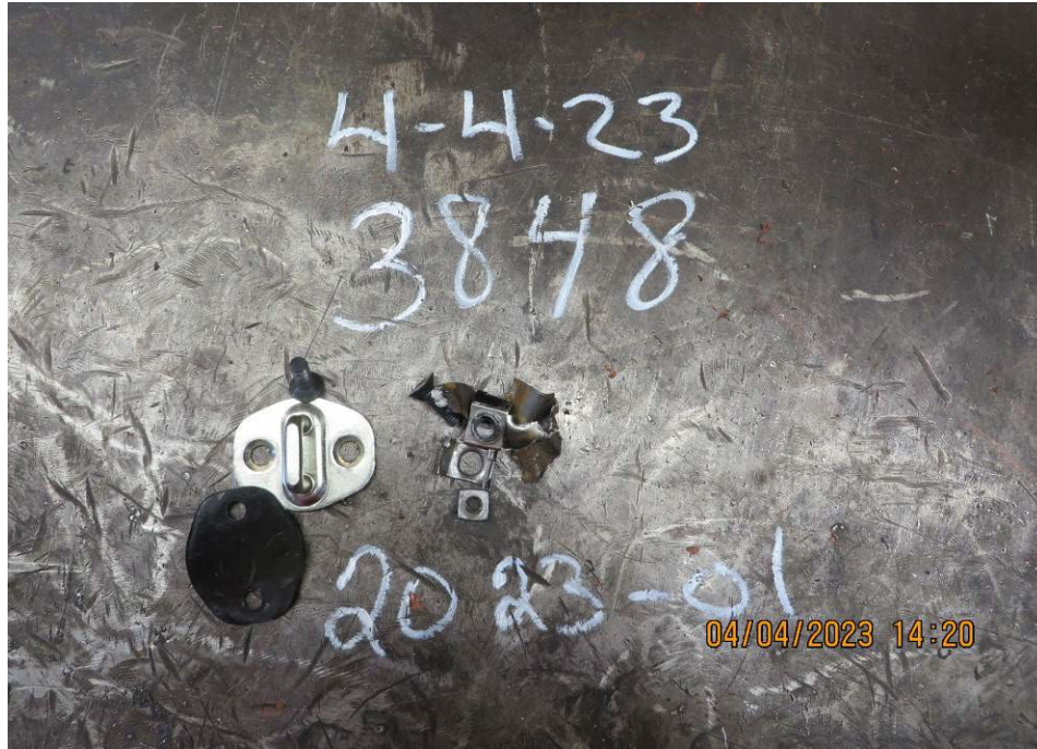
BROKEN REAR DOOR LATCH (3,701 TEST MILES)
