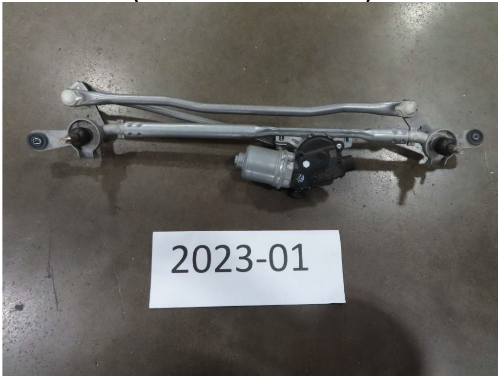
WIPER MOTOR REMOVAL AND REPLACEMENT (0.17 LABOR HOURS)
