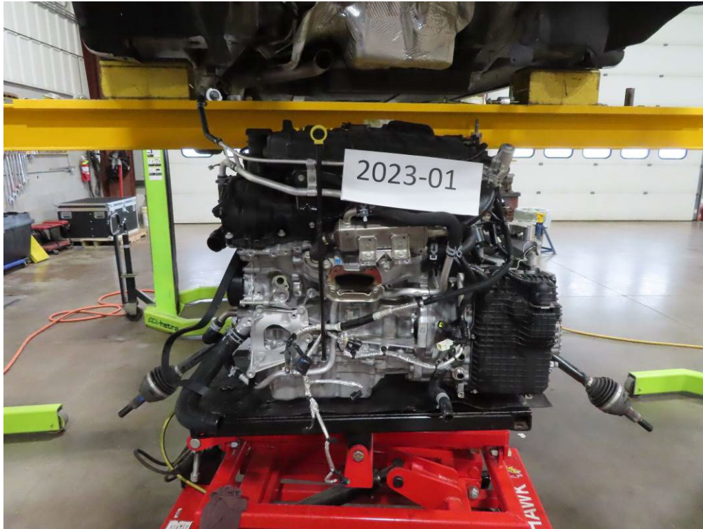
ENGINE/TRANSMISSION REMOVAL AND REPLACEMENT (8.00 LABOR HOURS)
