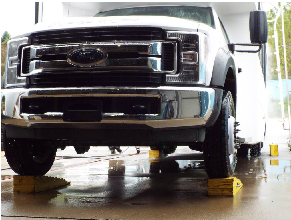
LEFT REAR WHEEL SIX INCHES LOWER
