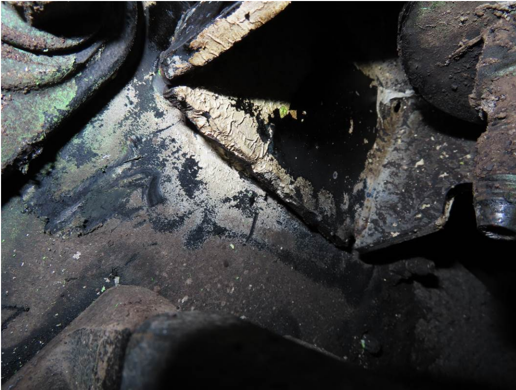
BROKEN BODY MOUNT WELD – FRONT OF REAR AXLE, LEFT SIDE (4,865 TEST MILES)
