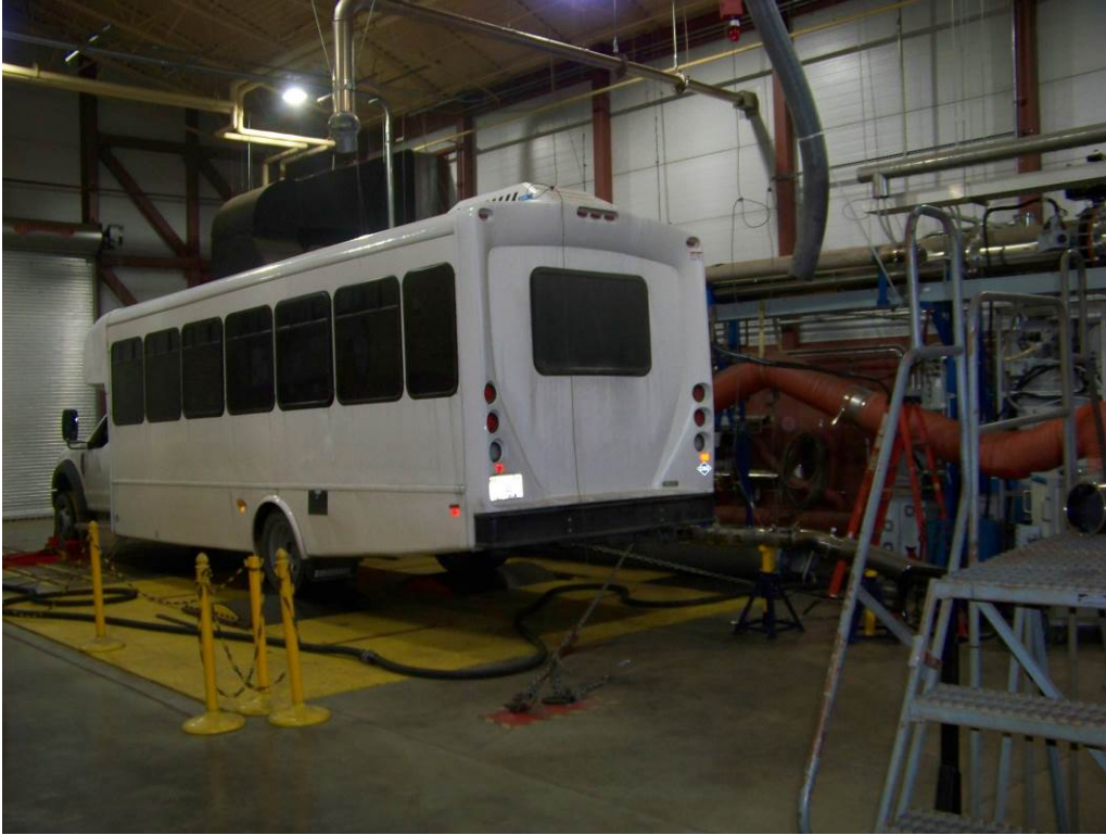
BUS TESTED ON CHASSIS DYNAMOMETER FOR PERFORMANCE, FUEL ECONOMY AND EMISSIONS
