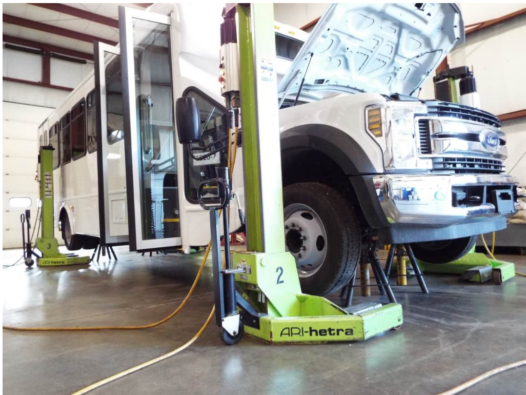
FRONT AND REAR OF BUS ON JACK STANDS
