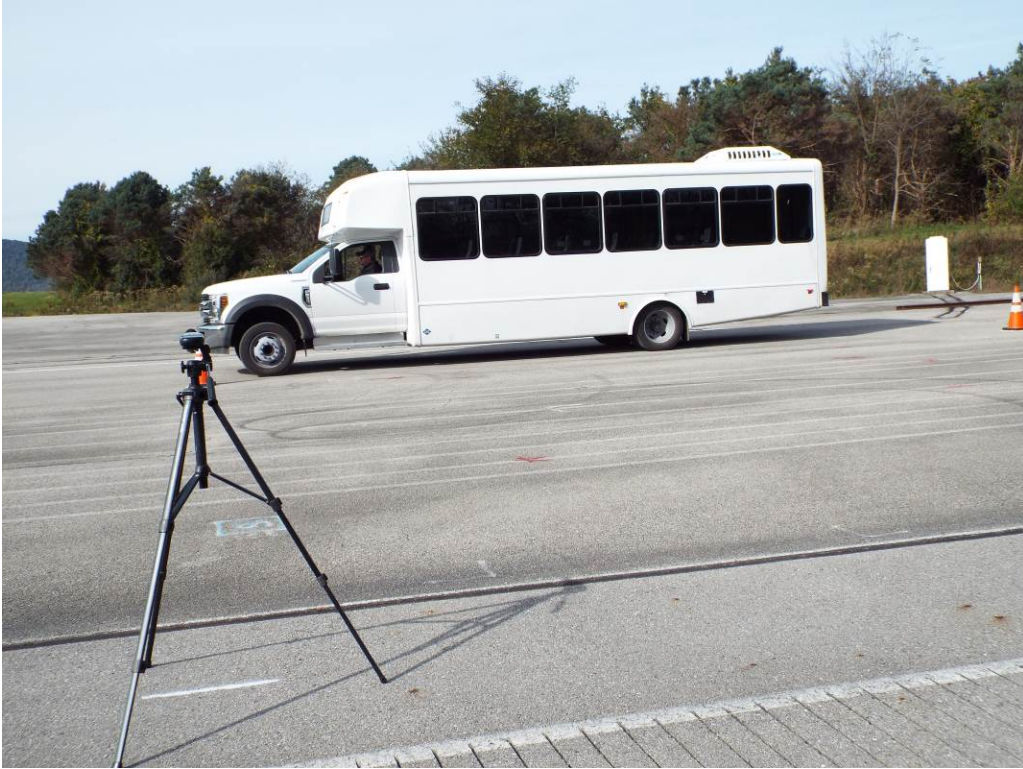
TEST BUS UNDERGOING EXTERIOR NOISE TESTING
