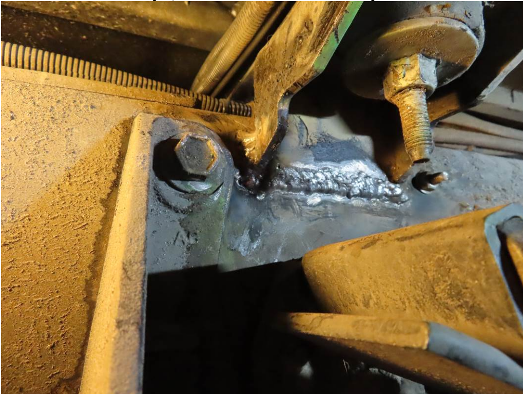
BODY MOUNT REWELDED – FRONT OF REAR AXLE, LEFTT SIDE (4,865 TEST MILES)
