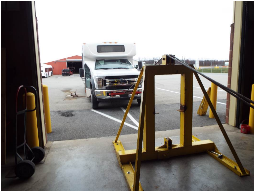
FRONT 20° UPWARD PULL
