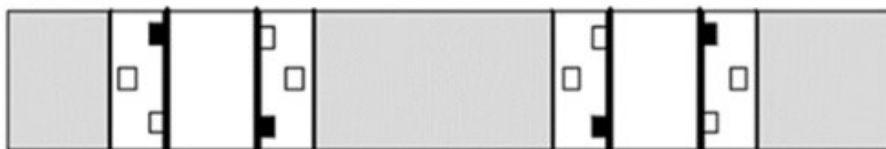
Figure A: Minimum acceptable spiking pattern
