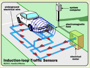
This graphic by www.HowStuffWorks.com shows the mechanics of an induction-loop traffic sensor.
