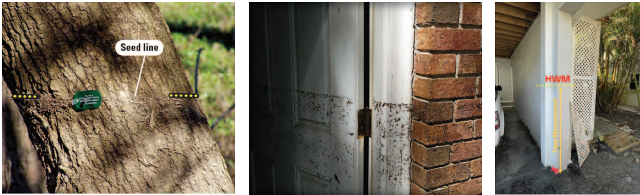
Figure 13: Seed Lines (Sources, left to right: USGS, USGS, Cotality)
