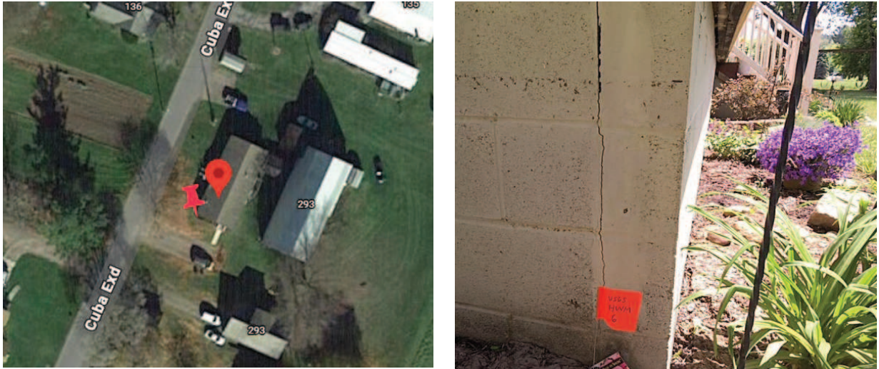
Figure 8: Example of Discrepancy Between GPS Location and Physical HWM Flag (Sources: Cotality and USGS)
