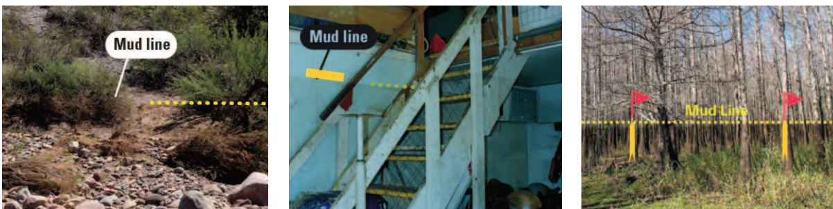
Figure 14: Mud Lines (Source: USGS)
