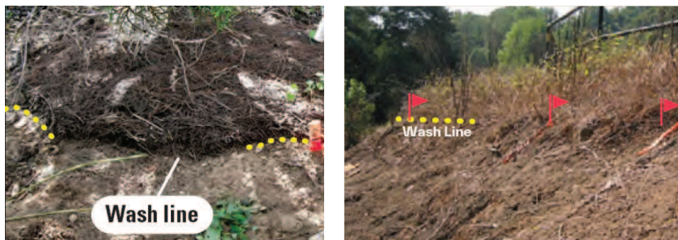
Figure 18: Wash Line Examples (Source: USGS)
