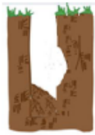
Closed Lip Failure
