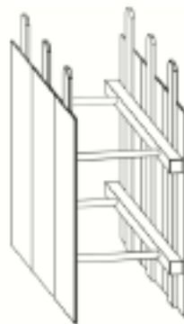
Panels, Struts and Wales
