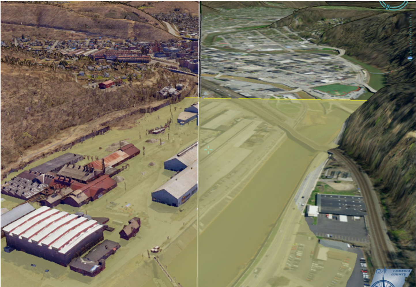
This image shows flood level analysis across both a 3D mesh on the left compared to traditional image draping on the right.
