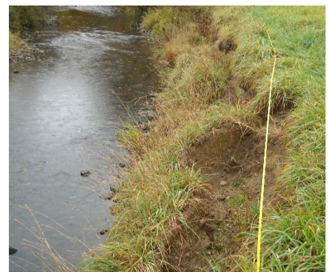
Top of the bank falling in due to the erosion at the toe-of-the-slope
