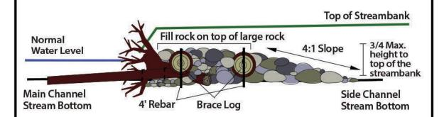
Note: Channel block built lower than surrounding streambanks while maintaining normal water level height
