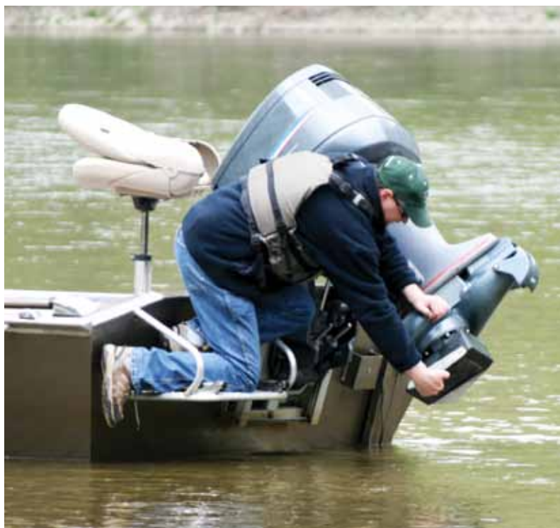
With an outboard jet drive, the water enters the bottom of the jet intake and is turned 180 degrees. It is expelled through the exhaust housing.
