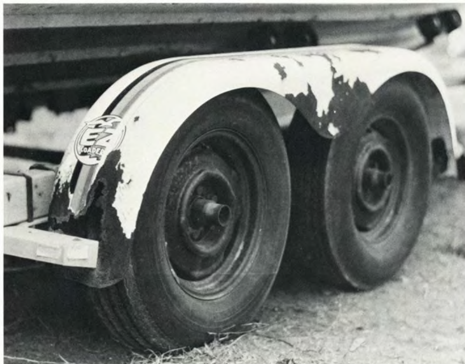
Rust is a trailer's constant enemy. A little preventive maintenance might have saved these boat trailer fenders. If your trailer is painted, be sure to touch up the paint job as needed. This could add years to the life of your trailer.
